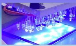
Figure 8. Testing the polymer curing time with UV LED bulbs.
