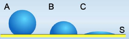
Figure 4. An example of varying droplet geometries and their contact angles with surface S; (A) large contact angle; (B) medium contact angle; (C) small contact angle
