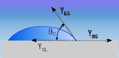
Figure 3. A liquid droplet on a substrate with interface angle labeled.
